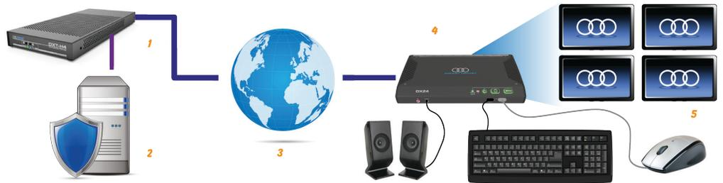
A DXT-H4 (1) connected to a closed host system (2) facilitates a remote desktop connection over a LAN/WAN (3) to a zero client (4) with quad video heads (5)
